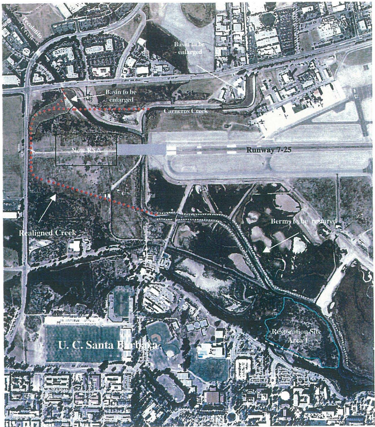
FIGURE 20 PROPOSED ENLARGED SEDIMENT BASINS
