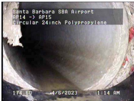
174.60ft Joint Angular Medium
