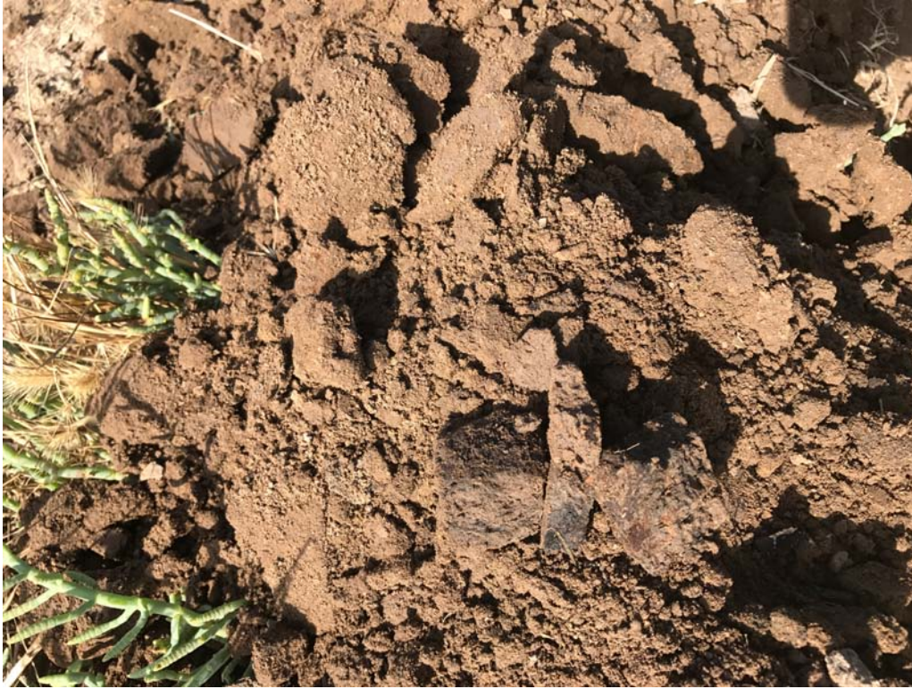
Photo 13. Soils at Data Point 3 showing fine sandy loam texture in upper 12 inches with darker clay horizon between 12-14 inches that forms an impermeable, restrictive layer.
